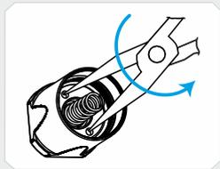
**!** Do not disassemble the flashlight except for unscrewing the thread ring gage and replacing the rubber button. There are no other parts in the flashlight that can be replaced by the user.
